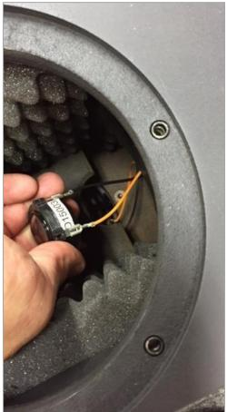
**STEP 4:** Carefully lift the non-functional Tweeter from the waveguide and extract it from the enclosure.
