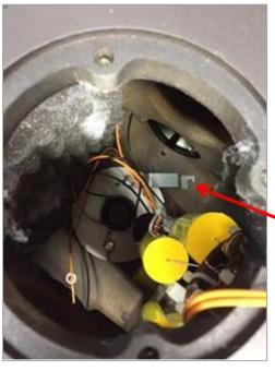
**STEP 3:** Loosen the wing nut so that you can move the bracket to one side.
